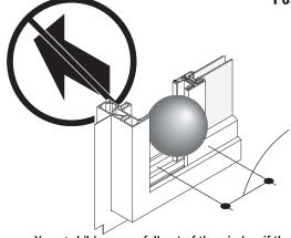
Less than 4" so that a rigid sphere can not pass through any space at the lowest opening portion in the window opening.
