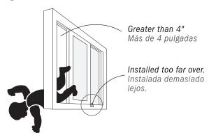
Young children may fall out of the window if the opening control device is not installed correctly. Install the device so that a rigid 4.0 inch (102 mm) diameter sphere does not pass through any space at the lowest opening portion in the window opening after the window opening control device (WOCD) is in place and engaged.
