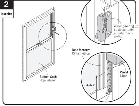
Verify correct side (left or right) to apply window opening control device. Measure up 3-3/4" from top of bottom sash meeting rail and mark on frame.
