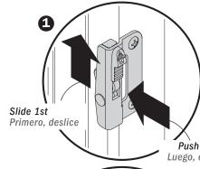
To fully open bottom sash, disengage window opening control device.
