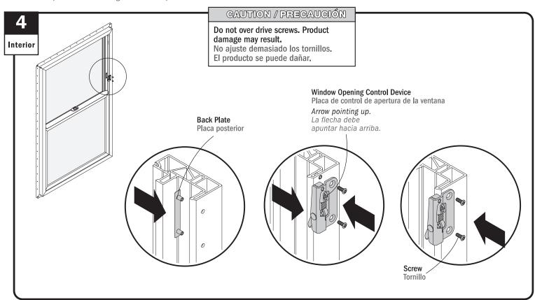
Position back plate to frame as shown. Position window opening control device at hole locations and fasten with 2 screws.
