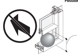
Less than 4" so that a rigid sphere can not pass through any space at the lowest opening portion in the window opening.
