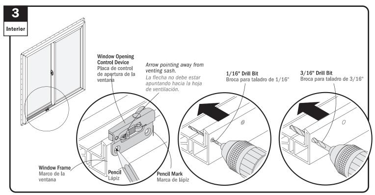
Position window opening control device tight to window frame on pencil mark. Mark hole locations and pre-drill 1/16" holes, as shown. Enlarge holes with a 3/16" drill bit.
