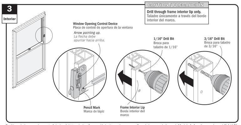
Position window opening control device tight to window frame with bottom edge on pencil mark (arrow pointing up). Mark hole locations and pre-drill 1/16" holes, as shown. Enlarge hole with a 3/16" drill bit. Remove drilling debris.
