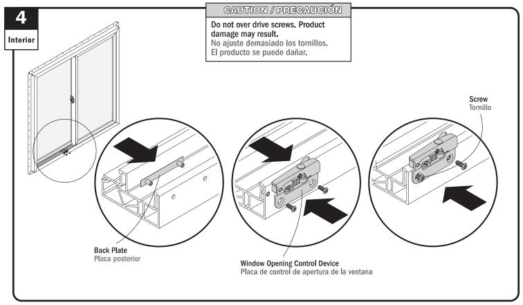
Position back plate to frame as shown. Position window opening control device at hole locations and fasten with 2 screws.
