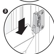
Lower bottom sash. Window opening control device resets automatically.
