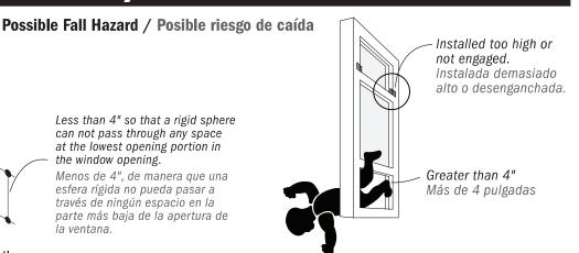
Young children may fall out of the window if the opening control device is not installed correctly. Install the device so that a rigid 4.0 inch (102 mm) diameter sphere does not pass through any space at the lowest opening portion in the window opening after the window opening control device (WOCD) is in place and engaged.
