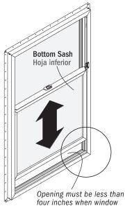
four inches when window opening control device is engaged.
